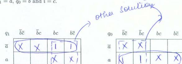
MSOP of  $q_1$  is  $\bar{a} \text{ or } b$
