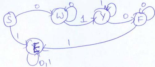
4. (15 points) Given the state transition diagram for a 1-bit input (a) draw the error state, E, for the missing inputs and (b) give the transition table.
