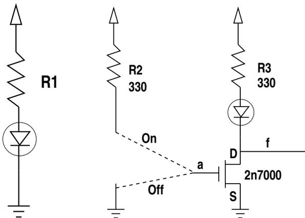
Figure 1: LED circuit
