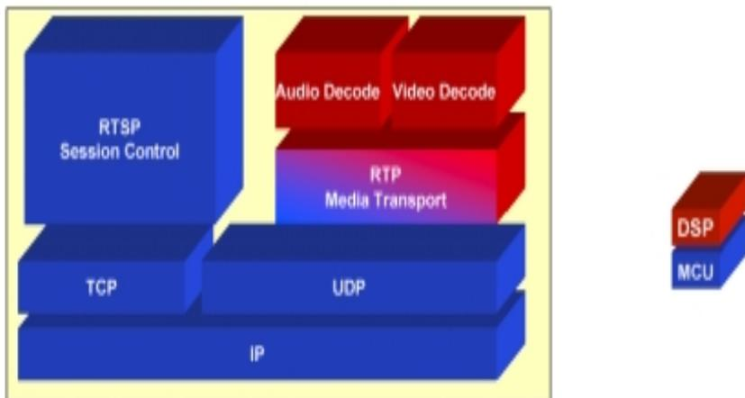
Figure 2: Partitioning of a Streaming Video Application
