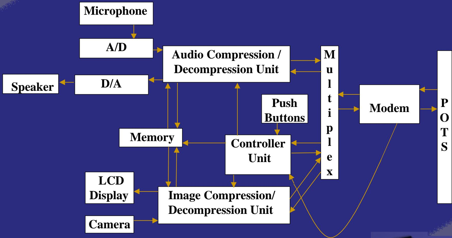
Figure 1 Block Diagram of the system components
