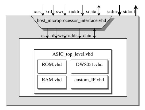
Figure 3: Microprocessor host test bench high-level architecture.
