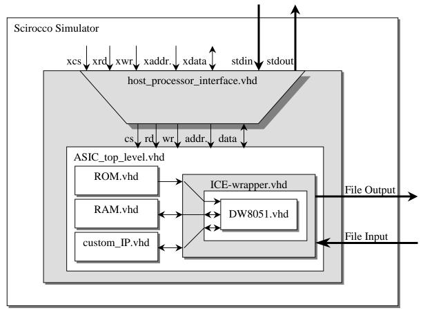
Figure 4: ICE test bench high-level architecture.
